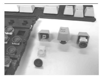
Figure 9. The architecture of a mechanical keyboard.
