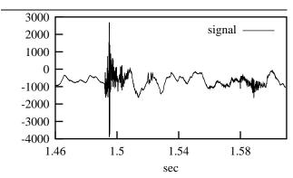
Figure 1. The acoustic signal of one click.
